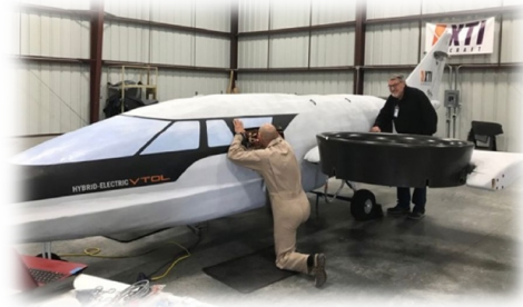
XTI 65%-Scale Proof-of-Concept Vehicle (2017–2020) Hover Tests
